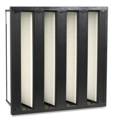
BioCel VXL<sup>®</sup> and AstroCel VXL<sup>®</sup> are lightweight compact filters designed for use in industrial HVAC installations. Available in the EN1822 classification range H10 - H13, their rigid design and pleated media pack with hot melt separators ensure they deliver the desired air quality when used as last stage filter in the AHU.
